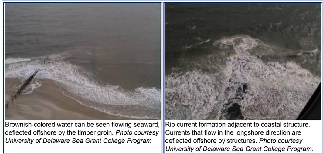
As waves approach the shoreline, they usually break at an angle, generating a longshore current that flows parallel (along) the beach. When the longshore current (moving along the shore) encounters coastal structure (such as a groin, jetty, or pier) it is deflected in an offshore direction. This offshore-directed flow of water is called a rip current.
