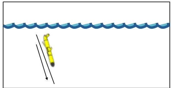
NOTE - Make sure the glider sinks nose first, not tail first. Also, you can make your water saltier if the glider is not sinking.
