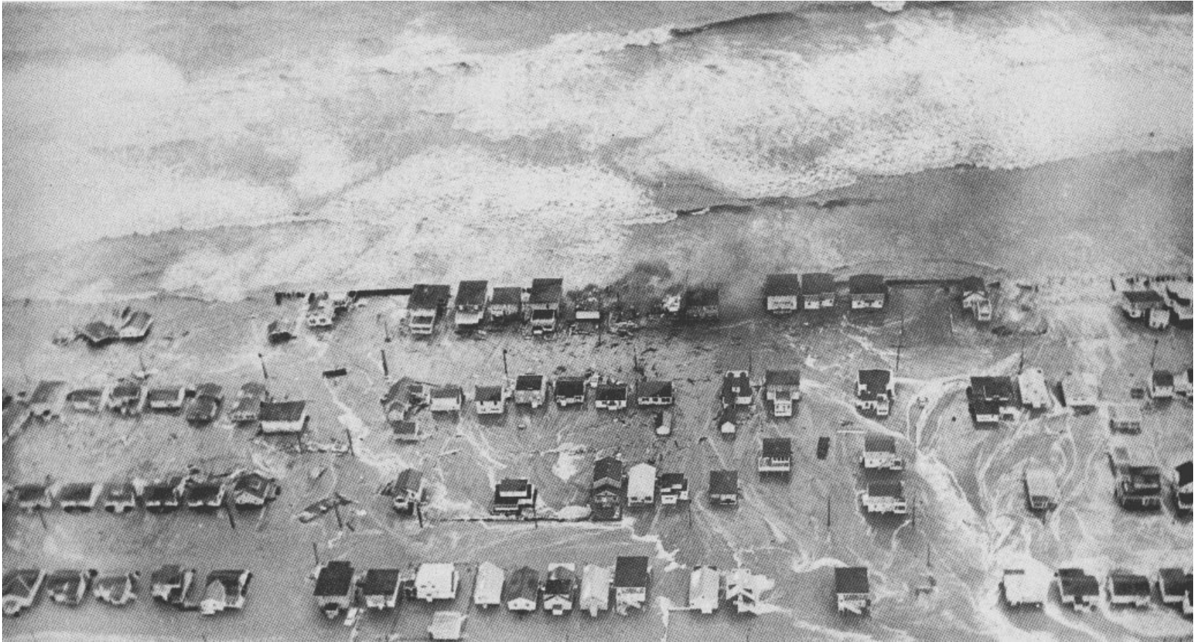
Ocean City, NJ. Note the transport of water across the island by waves
