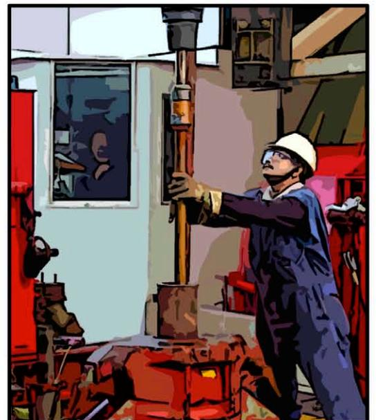
THE JOIDES RESOLUTION IS EQUIPPED WITH A POWERFUL DRILLING SYSTEM THAT LOWERS A DRILL BIT TO THE SEAFLOOR ON THE END OF A PIPE CALLED A DRILL STRING.
